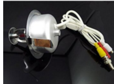
A CCTV camera that is installed inside a shell
