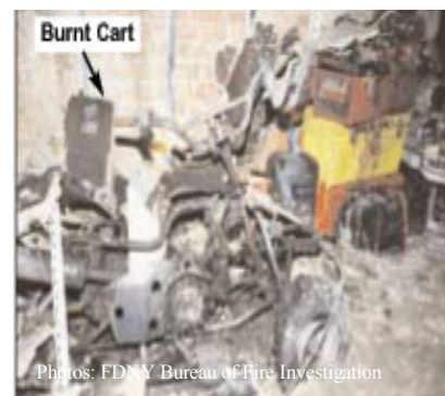
Fire was caused by gasoline and gas vapors escaping from the tank and ignited by the pilot light of the kitchen stove.
